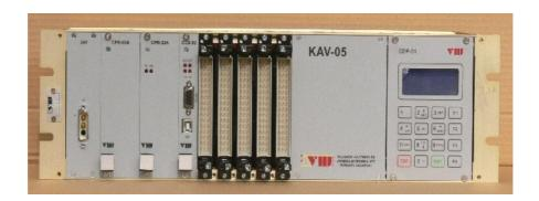
The coachmonitor KAV-05 supervises and controls the equipments of the railway coach. The main functions are as follows:
